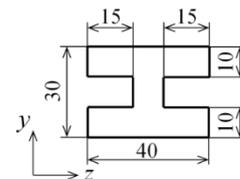
Figure 8 Shape of section
