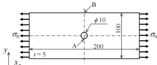
Figure 11 Exercises 3 (Flat plate with circular hole)
